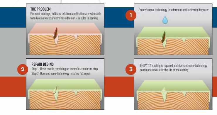
Encore's nano-chemistry is dispersed throughout the entire coating, and reacts with water in this way every time, whether the interaction is deep in a crack, or simply on the surface where there's no cracks at all. The proprietary technology lies resident in the coating, continually waiting for an opportunity to fortify weaknesses that appear in the coating over time.
