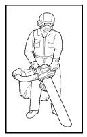
bag off elbow. Open other end of bag, and empty contents. Close bag, and reattach to blower. Secure bag with Velcro strap.
