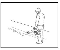
wide open throttle for at least 5 minutes every hour, and inspect/clean the spark arrestor screen after approximately 40 hours of operation.
