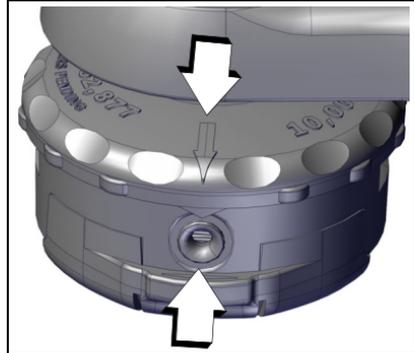
3. Insert one end of trimmer line into an eyelet, and push line equal distance through trimmer head.
