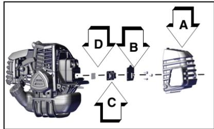
Note: When cleaning carbon deposit, be careful not to damage the catalytic element inside muffler.
