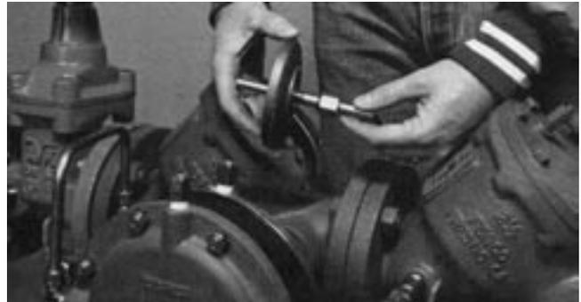
NOTE: On older Model 825 valves, the disc holder is sealed to the stem with a sealant. If the seal is broken, the stem and holder must be cleaned and new sealant applied. Newer valves, Models 825D and 825YD, use an o-ring so a sealant is not required.
