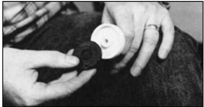
NOTE: The seat discs are symmetrical. It is usually possible to turn the disc over and obtain an effective seal.
