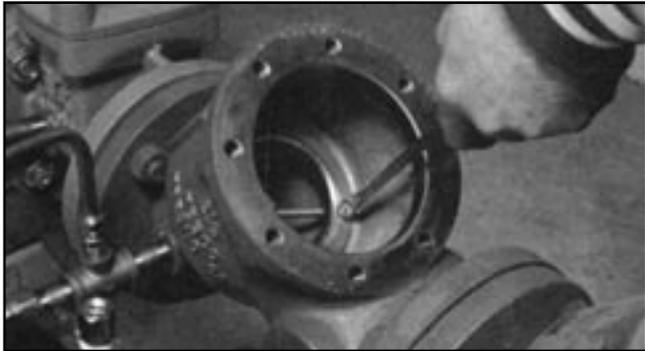
2. Pull the seat ring from the valve body being careful not to damage the internal epoxy coating of valve.
