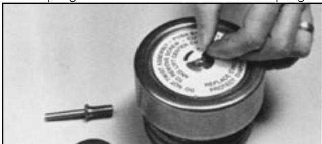
4. Remove the main stem and un-thread the retainer (Item 34) from the upper guide (Item 32). Remove the slip ring (Item 27a) and inner diaphragm (item 27). Inspect, clean and replace parts as required.
