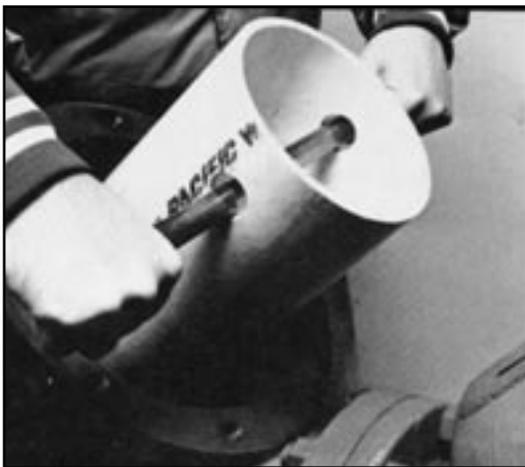
3. Remove bushing and bushing nut if used (bushing and nut is used on older Model 825).
