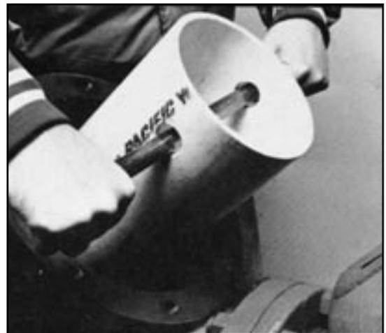
2. Remove bushing and bushing nut (item 2A & 2B).
