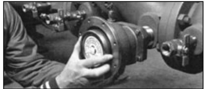
against the button. Work the rolled edge into the space between the module and the body making sure it is not pinched or buckled.
