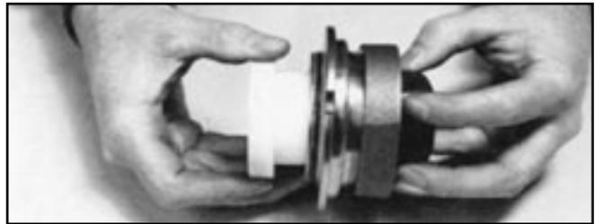
8. Once the inner diaphragm has been rolled, force the end of the main stem snug against the end of the inner diaphragm. The screw hole in the end of the main stem should be visible.
