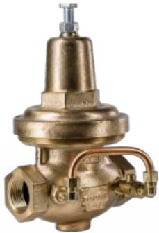
Reduces rapid pump cycle with field adjustable by-pass and maintains a pre-set operating downstream pressure for pump systems. Threaded female x female NPT connection with hex end OD. Features an unleaded body and cover. Nylon reinforced Buna-N diaphragm. Ideal for flows up to 70 GPM.
