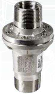
Reduces rapid pump cycling and maintains a preset system operating pressure independent from low or high flow conditions. Valve body is all stainless steel female NPT connection. The valve supports a hanging load up to 3,400 lbs. and fits in a 4" well casing.
