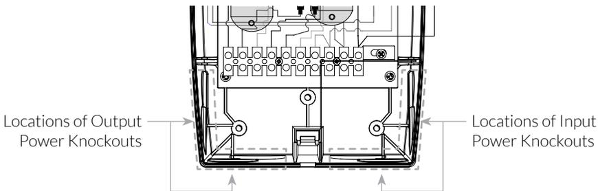
3. Using a hole saw, open the knockouts for the size of the conduit ( $\frac{3}{4}$ " or 1") being installed.
