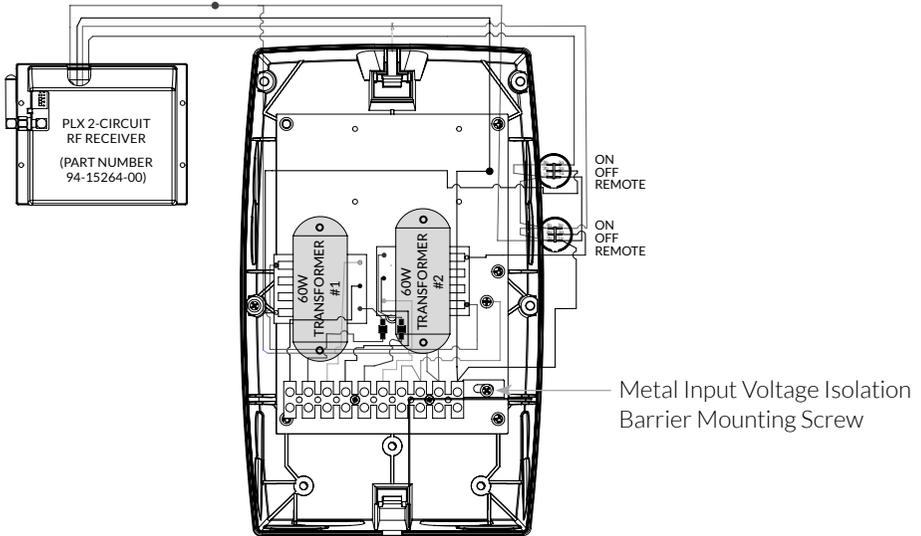
**\*Note:** Once all conduits are connected, replace the metal input voltage isolation barrier and mounting screw. Tighten until the mounting screw is secure.
