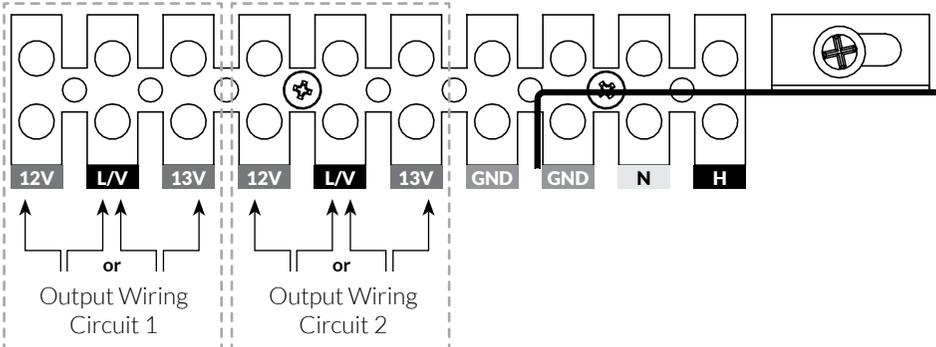
**\*Note:** DO NOT use or bridge both the 12VAC and 13VAC terminal positions at the same time.
