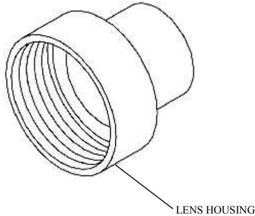
1. Cut the 1 1/2" pipe 1" back from flush to the wall (FIG. A). Remove any burrs from the pipe and glue the lens housing into the end (FIG. B and FIG. C). The LNS-2GI Lens Housing must be installed 12" to 14" down from top of wall.
