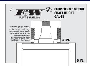
With the 024456 gauge resting at it's center point from the vertical motor shaft, the bottom edge of the appropriate motor diameter should clear the face of the motor.
