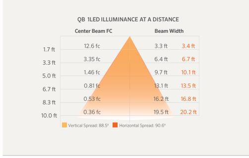
Beam angle is defined as two times the vertical angle at which the intensity is 50% of the maximum. It is calculated using LM-79 method for SSL Luminaires.
