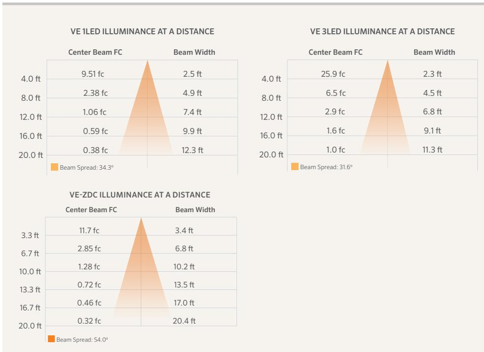
Beam angle is calculated using LM-79 method for SSL Luminaires:
