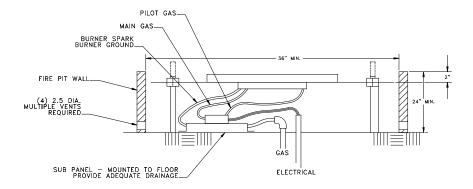
Figure 12: Propane Gas-Commercial Installation
