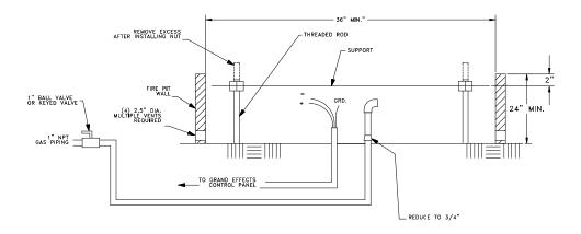
Figure 7: Propane-Commercial Installation
