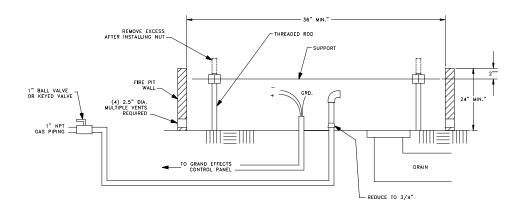
Figure 6: Natural Gas-Commercial Installation
