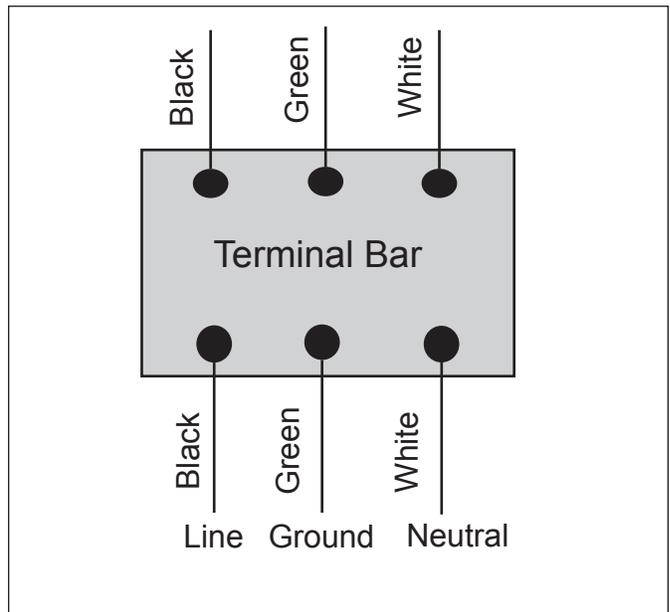
Figure 8. LX2 Factory Direct Wiring for 110 Volt Unit
