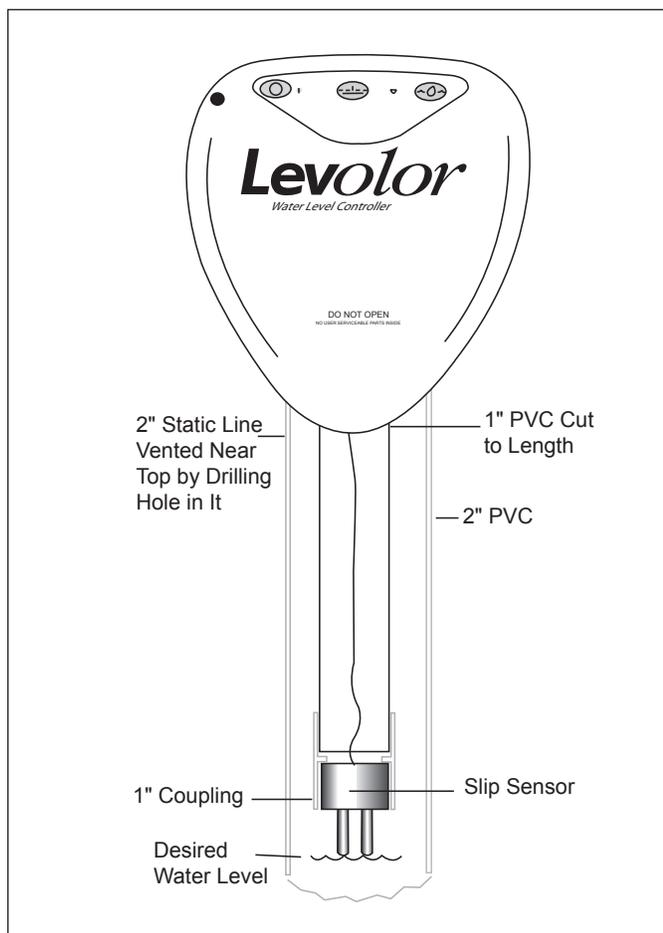
Figure 21. Slip Sensor in LX2 Installation Detail
