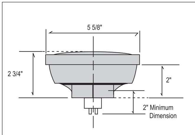
Figure 18. Slip Sensor in Remote Housing Detail
