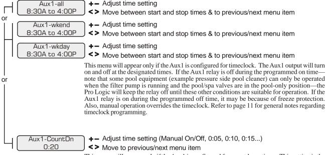
This menu will appear only if the Aux1 is configured for countdown timer. This setting is the time after you manually turn on the Aux1 relay until the Pro Logic automatically turns off the relay. You can also manually turn off the relay at an earlier time by pressing the AUX1 button.
