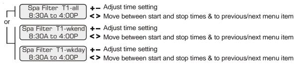
This menu is only available if the system has been setup for Dual Equipment. For one speed pumps, this is the first spa filter timeclock and will determine the normal hours of filtration for the spa. For pool/spa combination systems with spillover enabled, the valves will automatically switch to pool only at the start of the filtration period.
