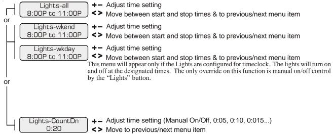
This menu will appear only if the Lights are configured for countdown timer. This setting is the time after you manually turn on the lights until the Pro Logic automatically turns off the lights. You can also manually turn off the lights at an earlier time by pressing the LIGHTS button.
