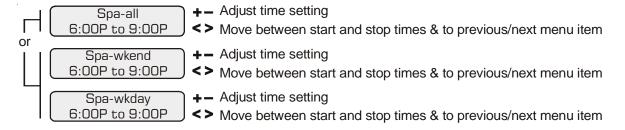
This menu is only available if the system has been setup for "spa only" or "pool and spastd". During the programmed spa time, the Pro Logic will move the pool/spa valves into the "spa-only" position and turn on the filter pump. The heater will automatically heat the spa up to the programmed spa temperature. This programmed spa operation will take precedence over all other automatic functions, only manual operation of the filter button or pool/spa valve button will override this function.
