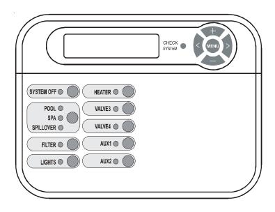
Optional Remote Display/keypad shown--the display keypad on the main control unit will have a "Service" button in the upper left corner instead of the "System Off" button.
