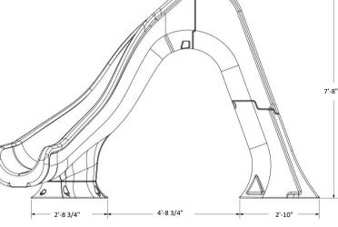
Height: 7' 8" Flume Length: 10' 11" Flume Width: 22" Required Deck Space: 11' 9" x 5' 5"
