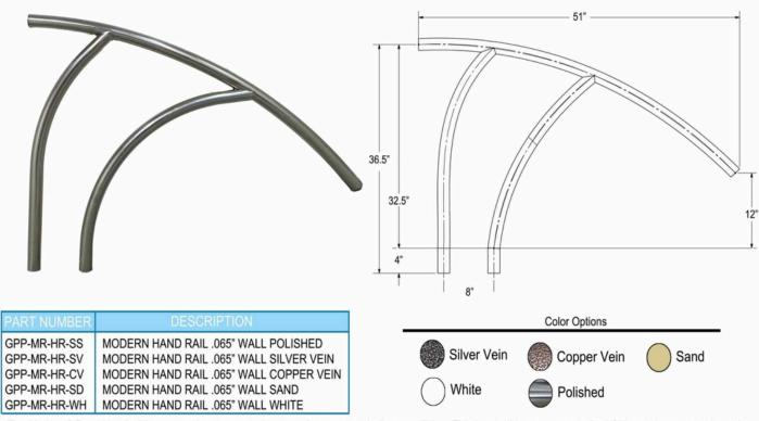
The Modern 3 Bend Handrail has several options to help customize your handrail to your liking. This handrail is constructed of a 1.90" stainless steel tube with optional wall thicknesses of .065, while having the color options of white, sand, polished or one of the premium powder coat colors that include copper or silver vein.
