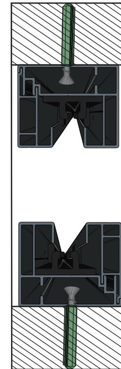
【Internal Installation】 : The roller curtain is mounted inside the frame and secured from the back of the track.
