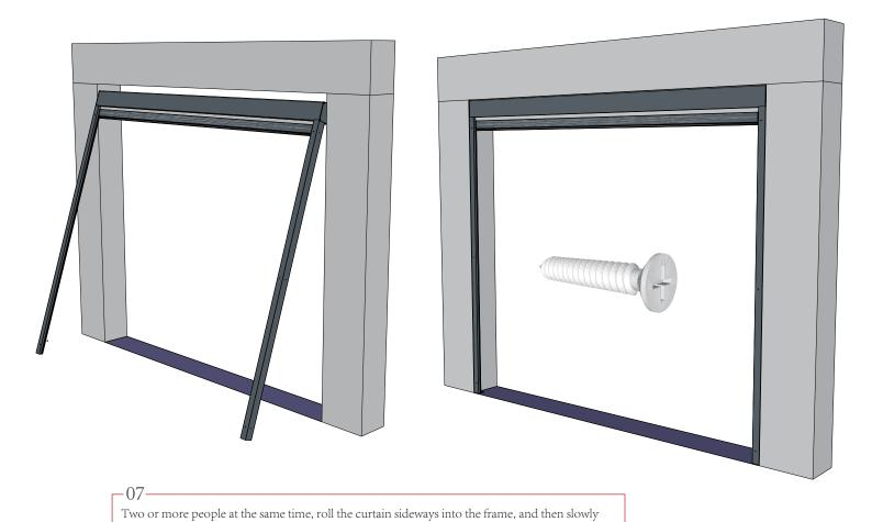
straighten until the curtain and the track fit into the frame, and then screw the track.
