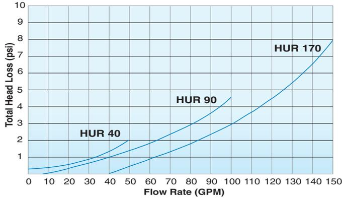
Pressure drop shown at left is for filter housing and 20 micron filter cartridge in clean water.
