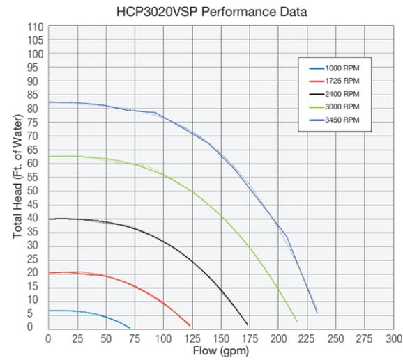
PUMP OUTPUT (GPM) VS. TOTAL RESISTANCE TO FLOW (PER FT OF HEAD)
