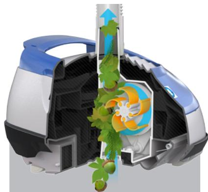
V-Flex Technology virtually eliminates clogs. As the turbine rotates clockwise, the variable vanes flex downward, allowing larger debris to pass easily.
