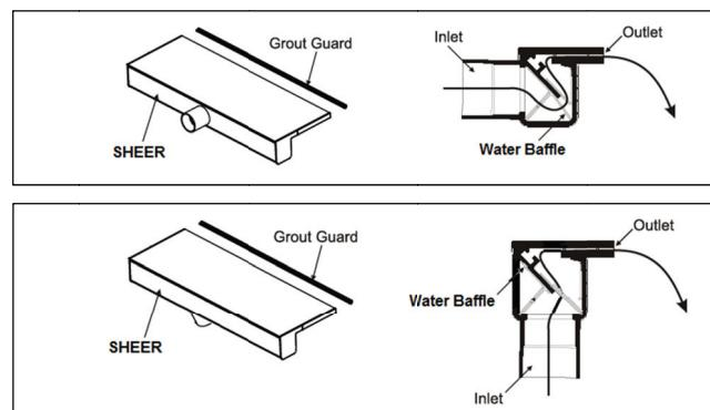
For multiple SHEERS, Hayward recommends that individual valves and lines be installed to allow balancing of the flow.
