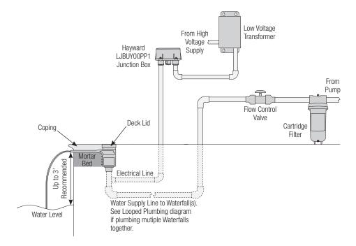
Refer to page 2 when determining the pipe size for the water supply line. Note that when using the optional rock trap (not pictured above), 2" plumbing is required.
