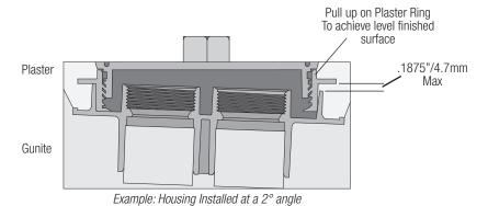
Apply and smooth out plaster around the edge of the plaster shield as seen below. The surface of the plaster should be even with the finished surface level.
