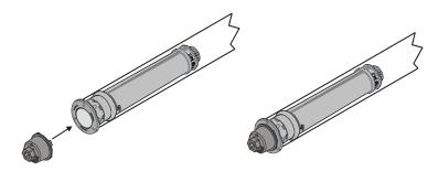
3) Slide the ring tool over the nut tool and insert tabs into the light face. Hold the nut tool with a wrench while rotating the ring tool clockwise. Handtighten the ring tool until snug. Do not overtighen.
