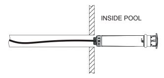
2) Insert the ColorLogic/CrystaLogic 1.5" LED light fully into the conduit. Insert the included hex nut tool into the 3 slots on the light face as shown.
