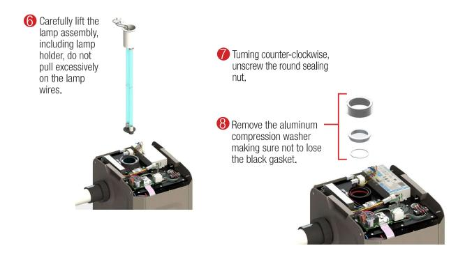
**NOTICE:** Do not touch the glass part of the lamp as body oils will create hot spots & greatly shorten lamp life. Inspect the quartz tube carefully for any cracks or chips and replace the quartz tube if any are found. Do not use any other O-ring for sealing the quartz tube. Never use any type of lube or sealing agent. Doing so can result in a leak and possibly damaging the UV unit.
