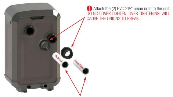
After cutting pipes to length, debur all cut pipe to ensure shavings don't plug critical points internal to the unit. Use PVC solvent cement to glue pipes into the union sleeve. NOTE the inlet and outlet pipe positions.
