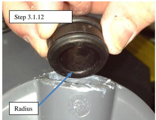
3.1.14 The liner has a definite orientation in the body. It is not symmetric from the top to the bottom. It is symmetric from face to face.
