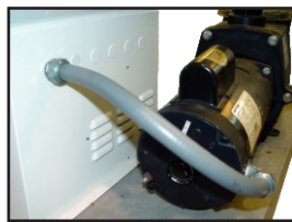
5) Route the other end of the conduit through the empty knock-out and secure with lock-nut. The cord inside will route up to the terminal strip inside the upper portion of the enclosure.
