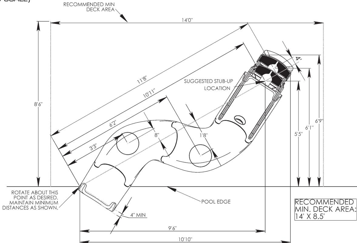
**SLIDE PLACEMENT DIAGRAM & FOOTPRINT DIAGRAM**
