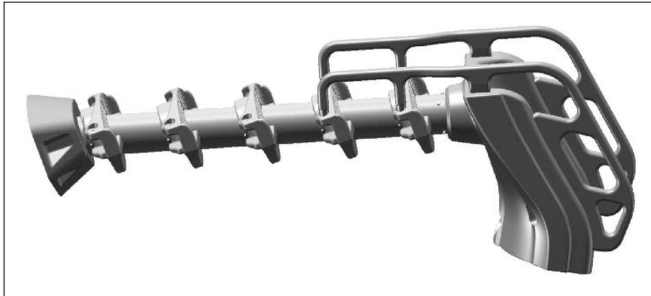
**Fig. 2: Ladder Step Support Sub-Assembly**
