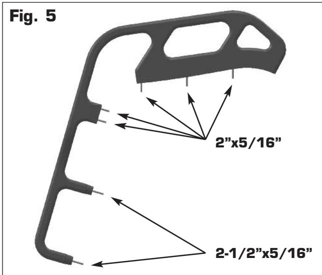
Hand tighten all-thread into each of the 7 locations on the handrails. Ensure correct length of all-thread is used at each location.
