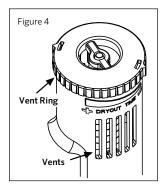
There is an adjustment capability on the Rain-Clik that will slow down the reset rate. By closing the "vent" (Figure 4) to completely or partially cover the ventilation slots, the hygroscopic discs will dry out more slowly. This adjustment can compensate for an "overly sunny" installation location, or peculiar soil conditions. Experience will best determine the ideal vent setting.
