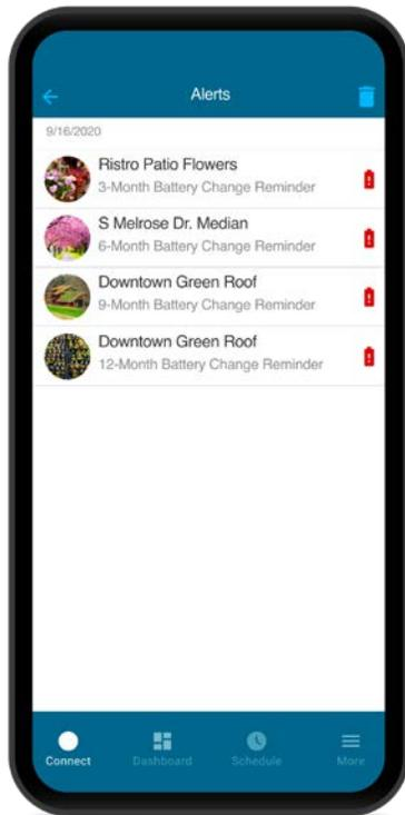
**DC controllers inevitably require periodic battery replacement.** With the NODE-BT App, you can easily recall maintenance records and note the last battery-change date. To ensure timely service intervals, you can set reminders to replace batteries at each controller every 3, 6, 9, or 12 months.
