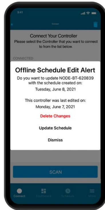
Speed up NODE-BT programming with preset schedules that are transferable to any controller in seconds. This ability reduces new controller setup time using preset Start Times, Run Times, and Water Day configurations for sites that have identical landscapes, allowing installers to bypass these steps and continue with other priorities. Preset schedules include custom-named stations and programs, Seasonal Adjust triggers, and Cycle and Soak settings.
