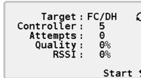
3. Use the OPTION
