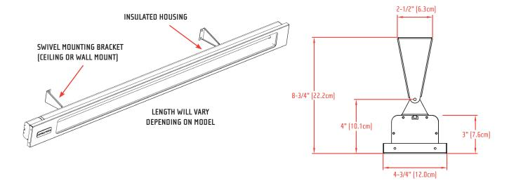
Heater must be installed with the quartz tube horizontally level. For maximum tube life, use a level to find the optimum position for the heater's body. Always maintain the minimum clearances from the heater body to any combustible materials.
