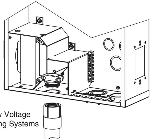
1. Install the Nonmetallic Hub to enclosure using Cable Clamp supplied.
