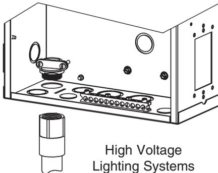
1. Install the Nonmetallic Hub to enclosure using Cable Clamp supplied.
