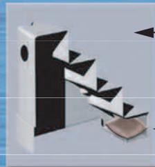
This cut-away view shows the inside of the step and ballast installation.
