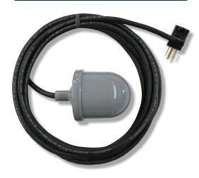
The Big Switch™ Pump Switch is used to turn a pump on and off in environments with temperatures up to 140° F. This product can be used for a variety of applications, including but not limited to: septic tanks, sump pits, holding tanks, pump chambers, water tanks, and any other liquid tanks. Available in 120/230VAC bare lead (no plug), 120VAC piggyback plug, and 230VAC piggyback plug, 15 Amp models.
