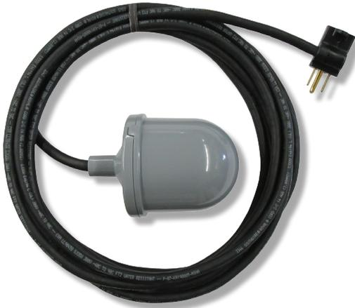
The Big Switch™ Pump Switch is used to turn a pump on and off in environments with temperatures up to 140° F. This product can be used for a variety of applications, including but not limited to: septic tanks, sump pits, holding tanks, pump chambers, water tanks, and any other liquid tanks. Available in 120/230VAC bare lead (no plug), 120VAC piggyback plug, and 230VAC piggyback plug, 15 Amp models.
