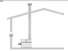
Figure 1-2\_Outside Combustion Air - Single Opening
