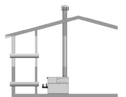
Figure 1-5\_Outside Combustion Air Through Ducts
