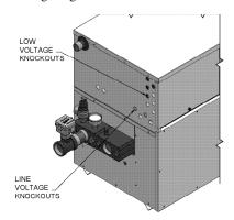
Figure 5-3\_Routing Field Wiring
