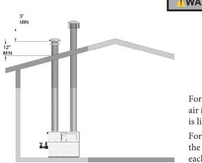
*Figure 2-8\_*Vertical DirectAire™ Installation *w*/Rooftop Combustion Air Inlet
