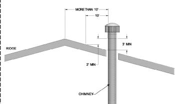
**Figure 2-2\_**Vent Termination from Peaked Roof - 10 ft. or More From Ridge
