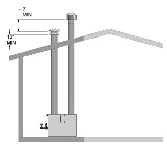
Figure 2-7\_Rooftop Combustion Air Inlet
