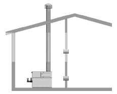
Figure 1-4\_Combustion Air from Interior Space
