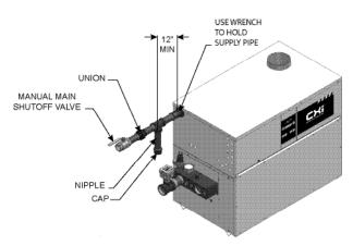
Figure 3-1\_Gas Line Connection
