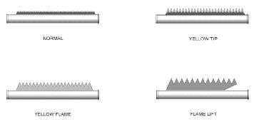
Normal Flame: A normal flame at 100% of burner input is blue, with slight yellow tips, a well defined flame and no flame lifting.
