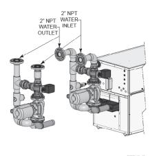
Figure 4-1\_Water Connections
