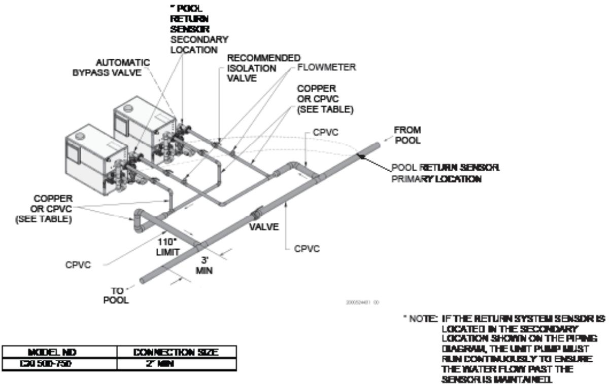
Figure 4-6\_ Cascaded Heaters Beyond 15 feet of Pool Piping
