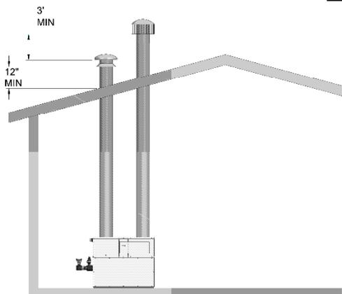
**Figure 2-8** Vertical DirectAire™ Installation w/Rooftop Combustion Air Inlet
