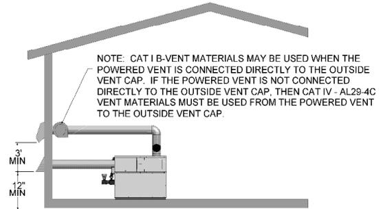
**B** This option uses a vertical conventional vent for flue products with air supplied by a pipe from the sidewall or rooftop - see page 18.
