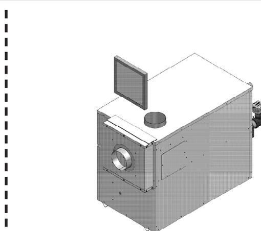
**Figure 2-12**\_Moving Air Filter Assembly & DV Box Adapter
