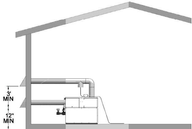
**C** This option uses a powered vent assembly to exhaust the flue products out a sidewall vent termination with air supplied from the equipment room - see page 21.
