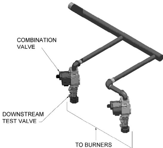
Figure 3-2\_Typical Pool Heater Gas Train Drawing
