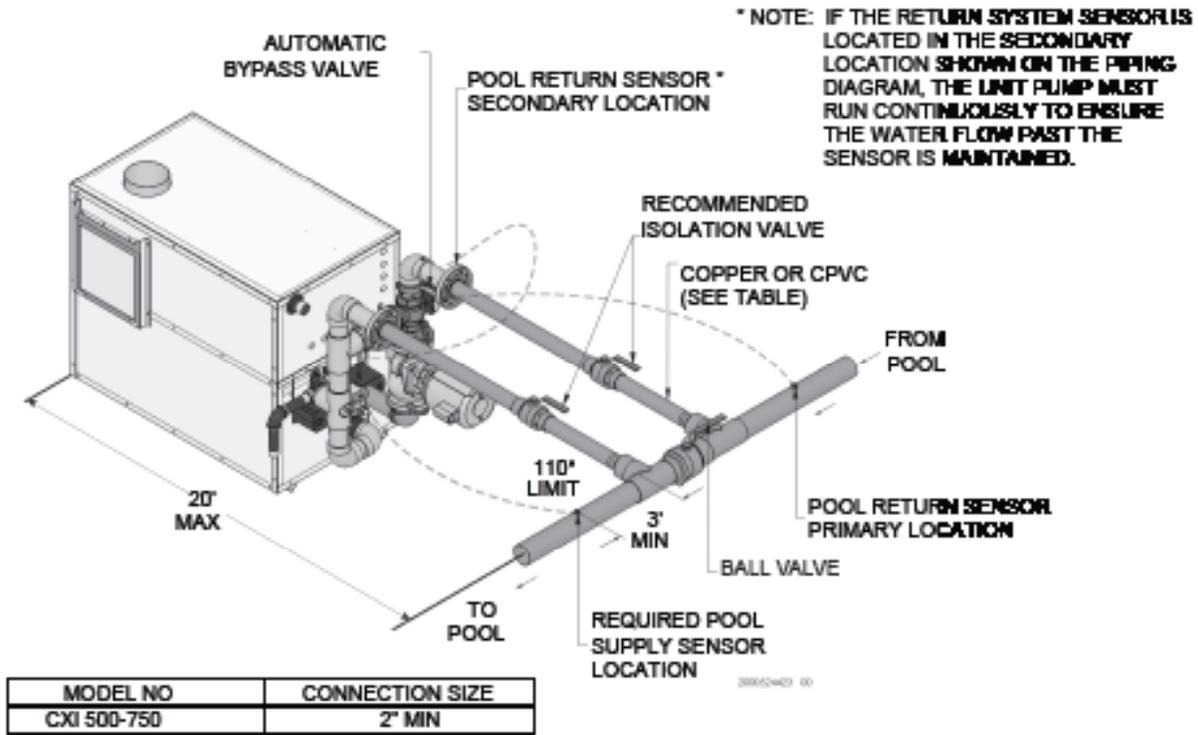
Figure 4-4 Heater Beyond 15 feet of Pool Piping
