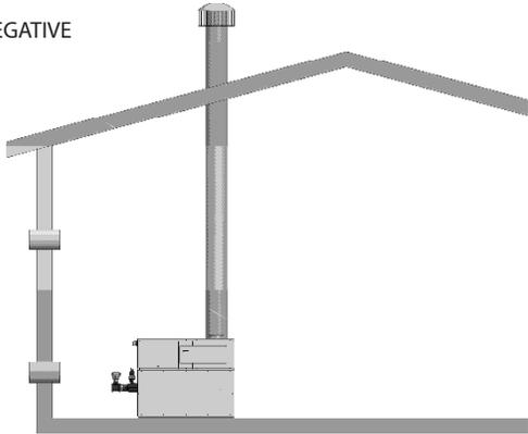
**D** This option uses a powered vent assembly to exhaust the flue products out a sidewall with air supplied by a pipe from the sidewall - see page 24.
