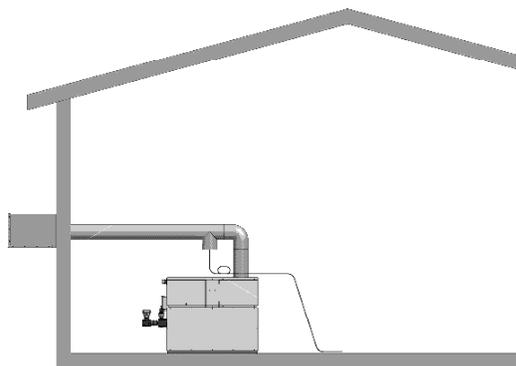
Figure 2-9\_Sidewall Vent
