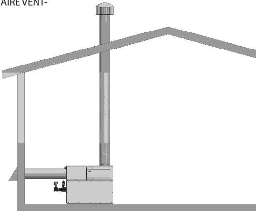
**E** This option uses a sealed AL29-4C flue and a separate combustion air pipe to the outdoors. This system terminates both the flue and combustion air inlet in the same pressure zone - see page 25.
