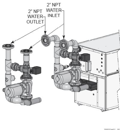
Figure 4-1\_Water Connections
