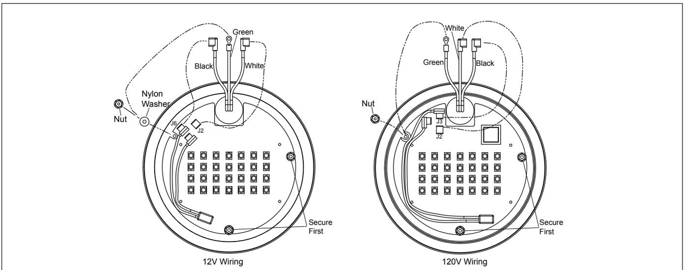
**Figure 3. Large Light Engine (PCB) Replacement and Wiring**
