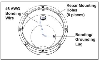
Figure 6. Stainless Steel Niche Bonding Wire Installation
