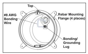
Figure 3. Plastic Niche Bonding Wire Installation
