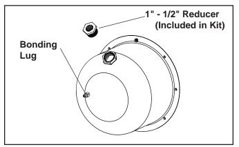
Figure 5. Stainless Steel Niche Kit Components
