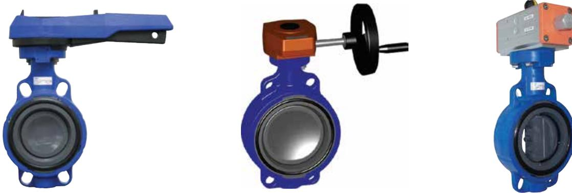
Specifically for water applications, the Type 563 Aqua butterfly valve operates at pressures of up to 150 PSI and can handle temperatures from 32°F to 142°F. The wetted inner body is made of PVC with EPDM seals. Because of the plastic body, the Aqua valve is lightweight and installs easily between flanges. The Aqua valve is compatible with ANSI and DIN flanges and is
