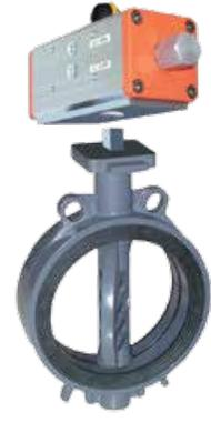
The VFA butterfly valve is Georg Fischer's economic solution for medium and lower duty applications. The valve is made of durable PVC and its light weight is a good fit for systems already incorporating plastic pipe and fittings. The disc seal is separate from the flange seal, reducing torque requirements.
