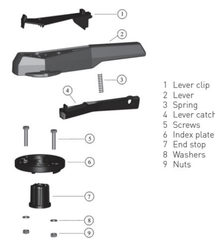
1. Hand lever should be assembled with disc closed. By the indication of the shaft and the end stop a clear assembly is ensured.
