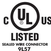
UL Listed as a Sealed Wire Connector. For use in dry, damp, wet locations below or above grade when used in an enclosure. For use in direct bury applications when operating at 30 volts or less.
