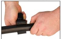
**SLIP** saddle onto pipe BEFORE LATCHING.
