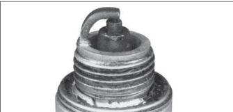
A wet plug is caused by excess fuel or oil in combustion chamber. Excess fuel could be caused by a restricted air cleaner, a carburetor problem, or operating engine with too much choke. Oil in combustion chamber is usually caused by a restricted air cleaner, a breather problem, worn piston rings, or valve guides.
