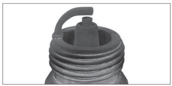
Soft, sooty, black deposits indicate incomplete combustion caused by a restricted air cleaner, over rich carburetion, weak ignition, or poor compression.
