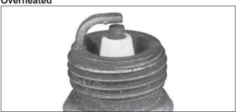
Chalky, white deposits indicate very high combustion temperatures. This condition is usually accompanied by excessive gap erosion. Lean carburetor settings, an intake air leak, or incorrect spark timing are normal causes for high combustion temperatures.
