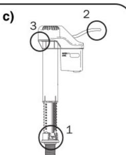
Do not use sealant / tape. **Hand-tighten only.** Parts may be left over.
