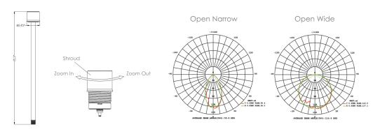
Construction: Brass Finish: Antique Brush Lead Wire: 6ft long Mounting: LAP-002
