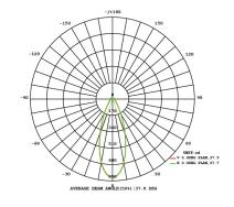
Construction: Brass Finish: Antique Brush Beam Spread: 38°
