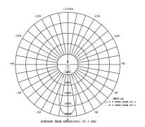
Construction: Brass Finish: Antique Brush Beam Spread: 35°
