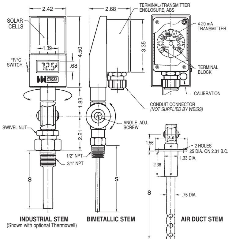
Compatible with most Building Automation Systems with 4-20mA input.
